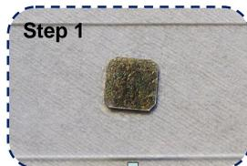
Step 1: Film is attached to a glass slide by wax
