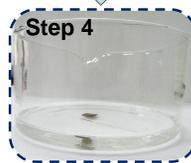
Step 4: Immersed in acetone for 12 h to dissolve wax.
