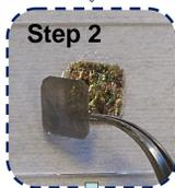
Step 2: Substrate thickness is reduced to 100 μm.
