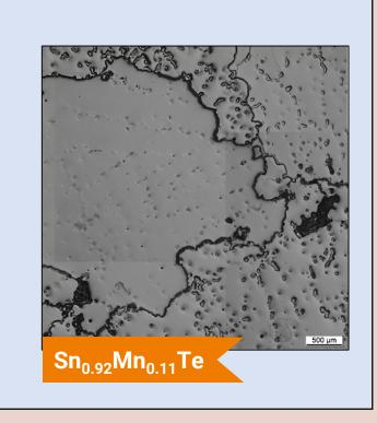
Very large grain sizes (diameters) of up to 2 mm → high ordering tendency
